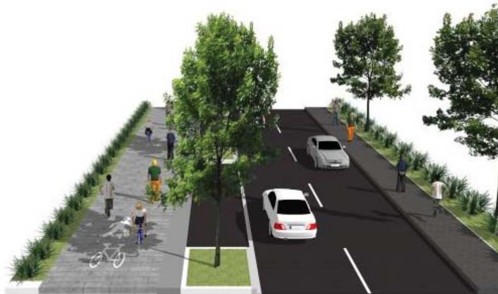
2.5-3m shared walkway/cycleway / 1m flush safety strip / parking and planting / carriageway / footpath
