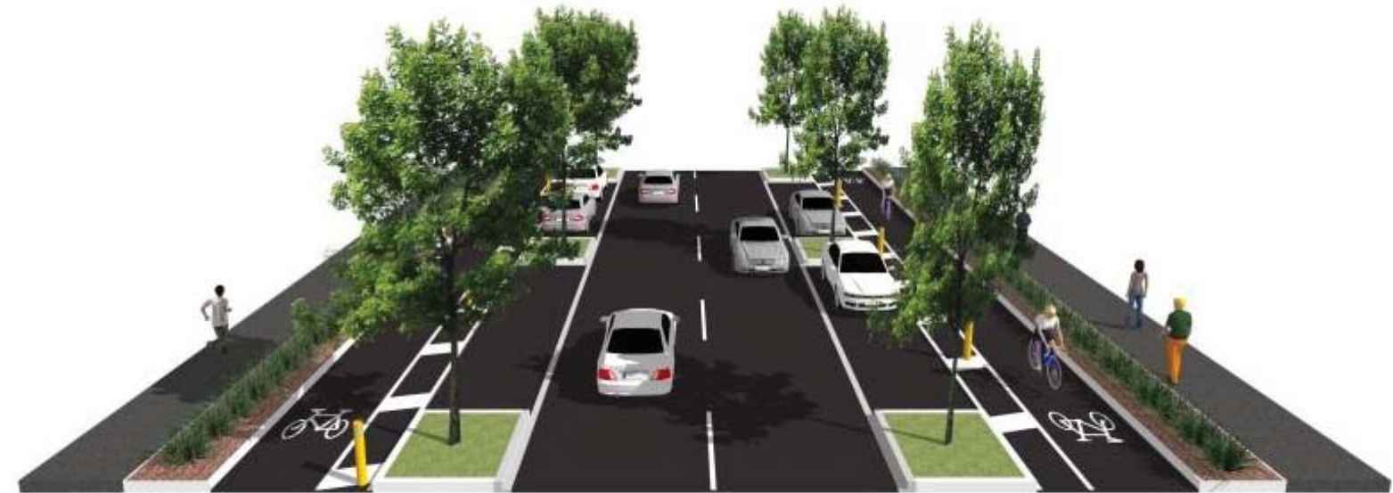
footpath / swale / one way cycle / 1m safety strip median / parking and planting / carriageway
