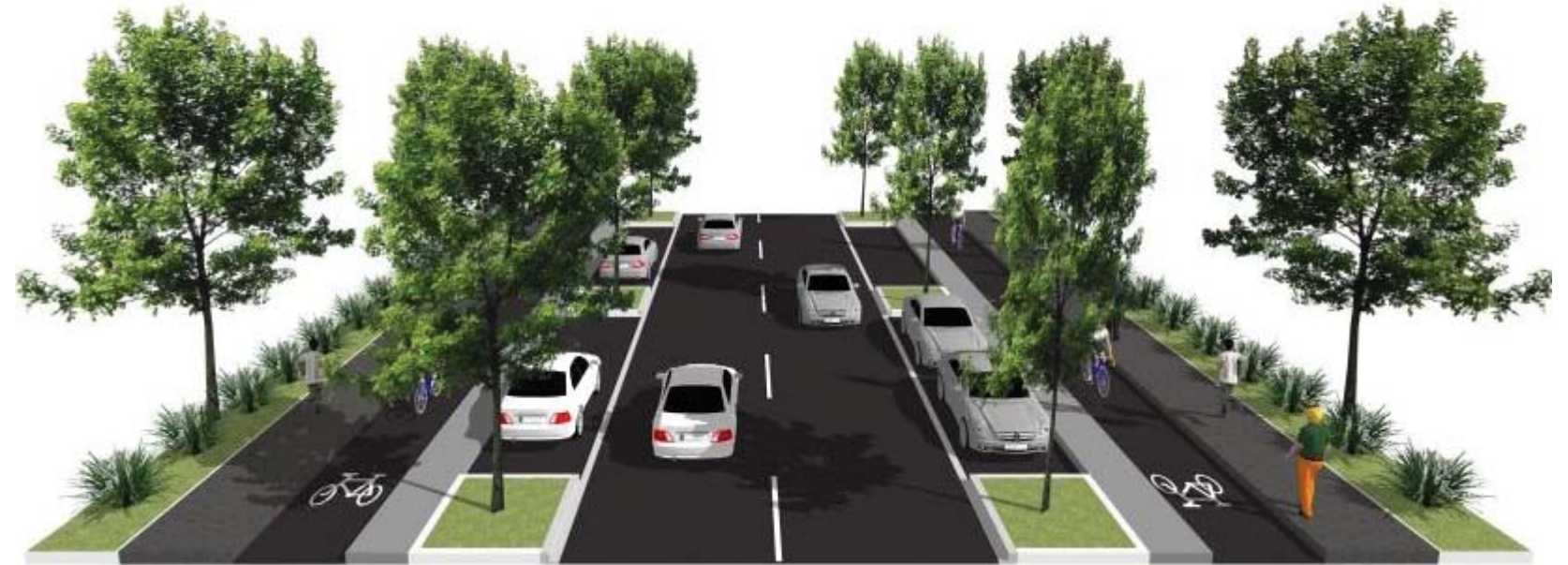
footpath and cyclelane (kerb as division) / 1m raised safety strip / parking and planting / carriageway
