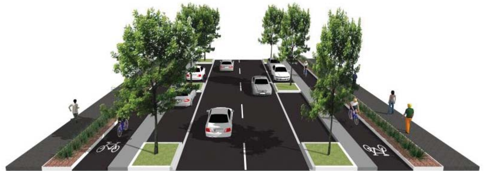
footpath / swale / one way cycle / 1m raised safety strip / parking and planting / carriageway
