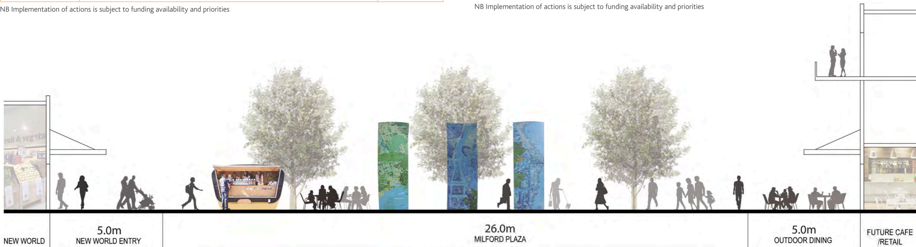
Figure 10. Indicative Milford Plaza cross-section, showing active frontages to each side (note dimensions do not indicate final design)
