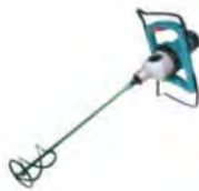
Single mixer with spindle paddle small quantities
