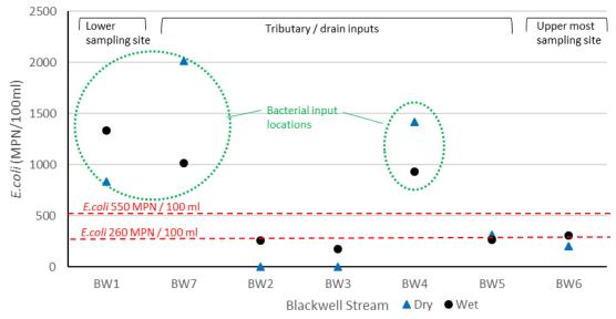
Figure 5. *E.coli* concentrations at Blackwell Stream, taken during March "Dry" and May "Wet" weather conditions 2017. Red dashed lines indicate guideline for recreational water quality (alert 260 and action 550 MPN/100ml; MoH/MfE 2003).
