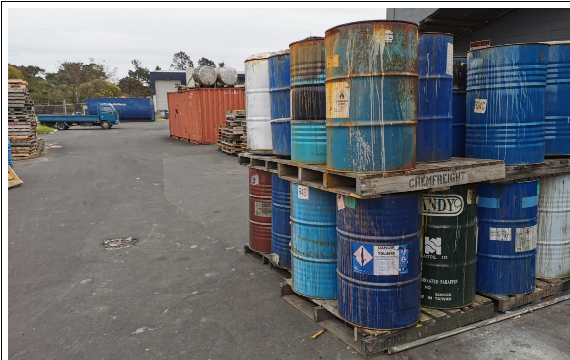
Photo above: This company was prosecuted for a spill at their site in Onehunga (now closed) when a 1000L container of paint spilt and got into the local stream. They also have significant risks at their East Tāmaki site. Large volumes of hazardous liquids are being stored outside in drums in poor condition, stacked on each other and without secondary containment. This site was immediately passed onto the council's compliance team following our visit in March 2020.
