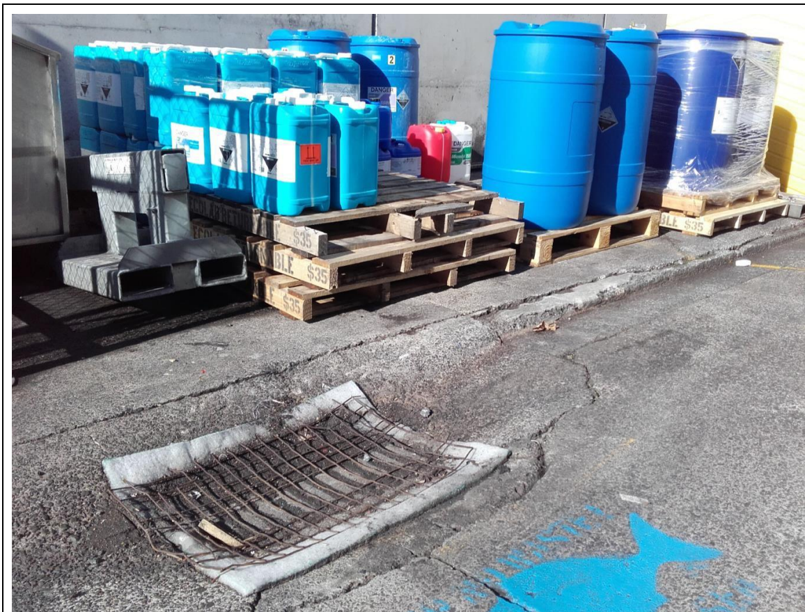
Photo above: Class 8 Corrosive liquids stored outside without any containment, next to a stormwater drain. The company is working on our recommendations to better store these chemicals. We will continue to follow up with them.
