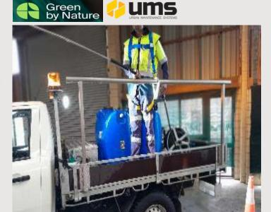
Outfitted the rear section of our waterblasting ute with sturdy safety rails
