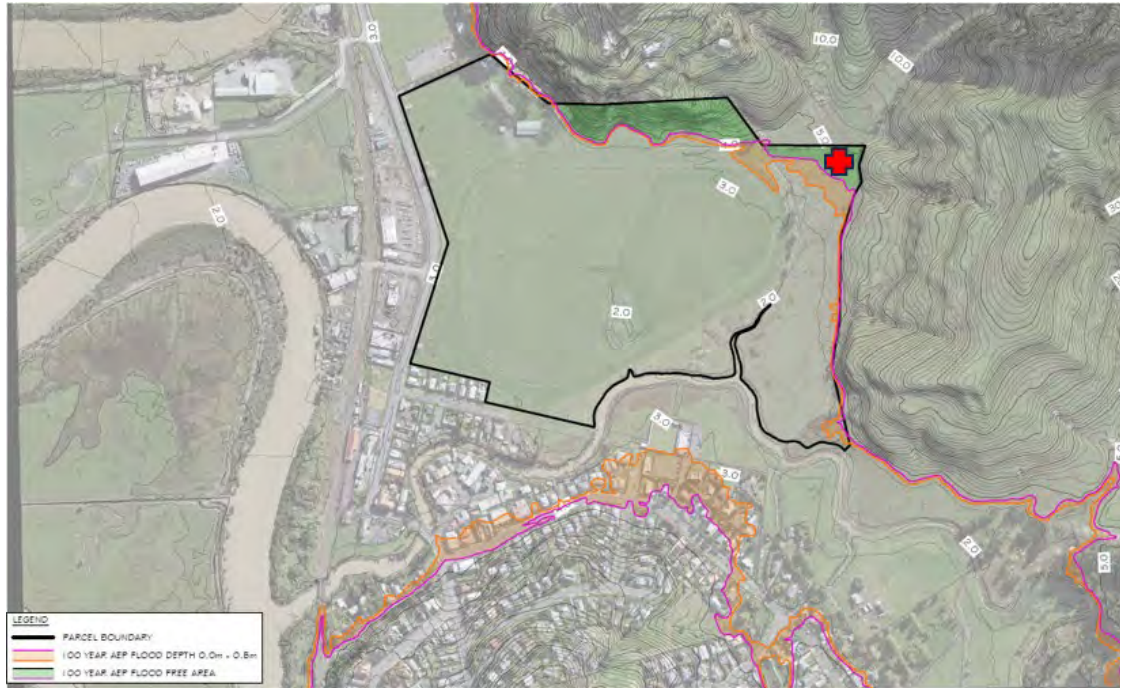
Figure 2: Updated floodplain plan with 100-year annual exceedance probability (AEP) showing flood free area shaded green
