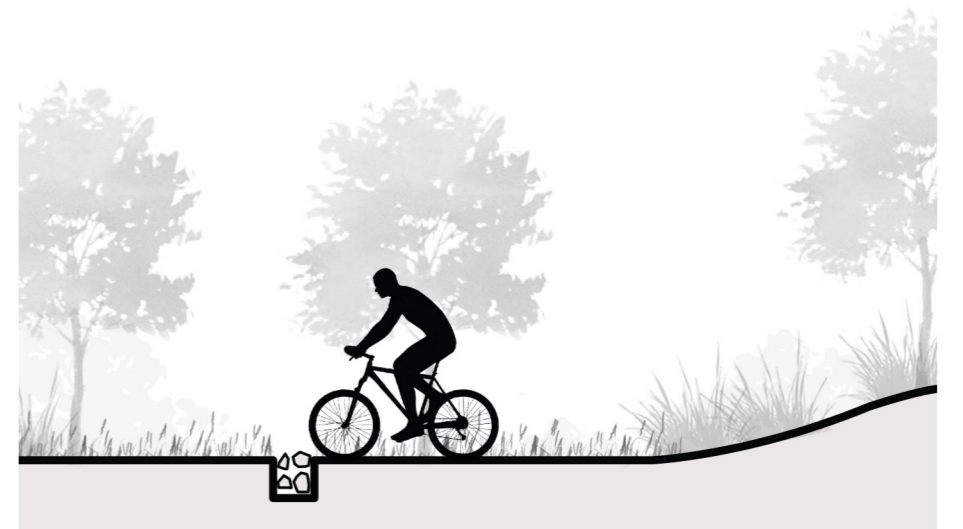
Riprap or Box Channel Drainage Crossings (.5m)
