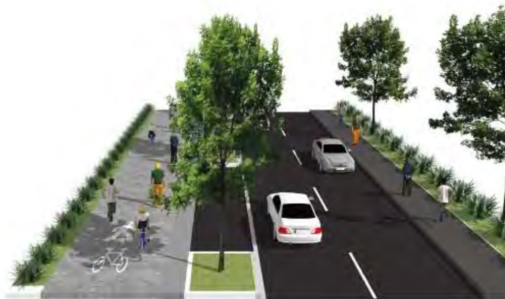
2.5-3m shared walkway/cycleway / 1m flush safety strip / parking and planting / carriageway / footpath
