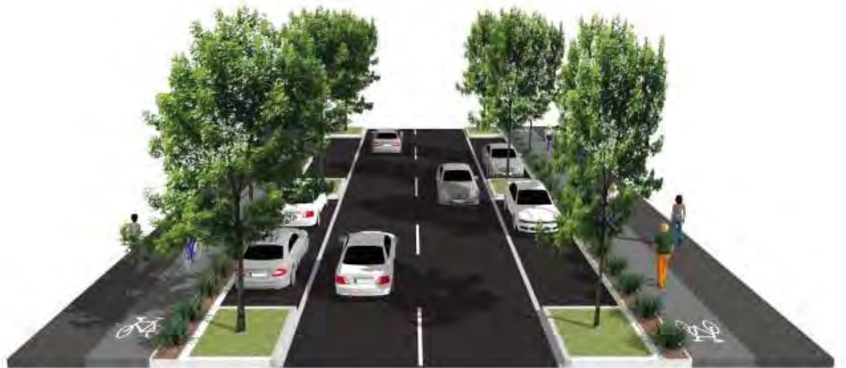
2.5-3m walkway/cycleway with marked division / planted safety strip / parking and planting / carriageway
