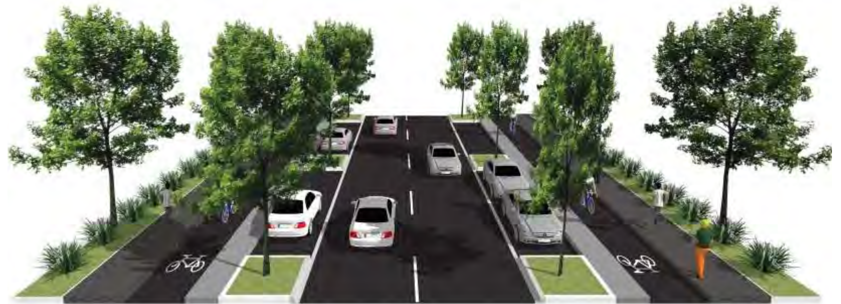
footpath and cycleway (kerb as division) / 1m raised safety strip / parking and planting / carriageway
