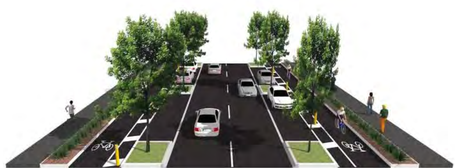
footpath / swale / one way cycle / 1m safety strip median / parking and planting / carriageway
