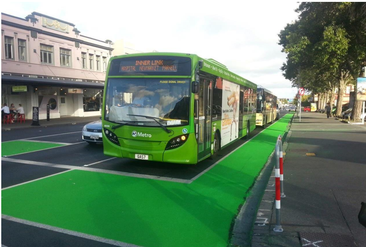
New cycle feeder lanes and advance stop boxes on Ponsonby Road.
