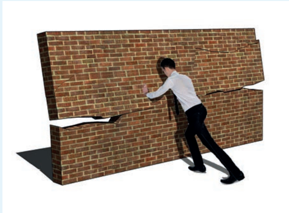
(a) Schematic of a wall responding out-of-plane.
