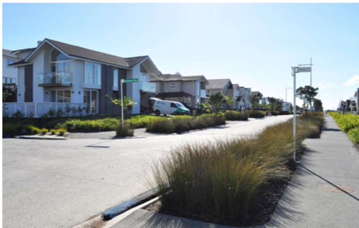
Figure 8: A green streets approach to roading in Long Bay (source: Auckland Design Manual)
