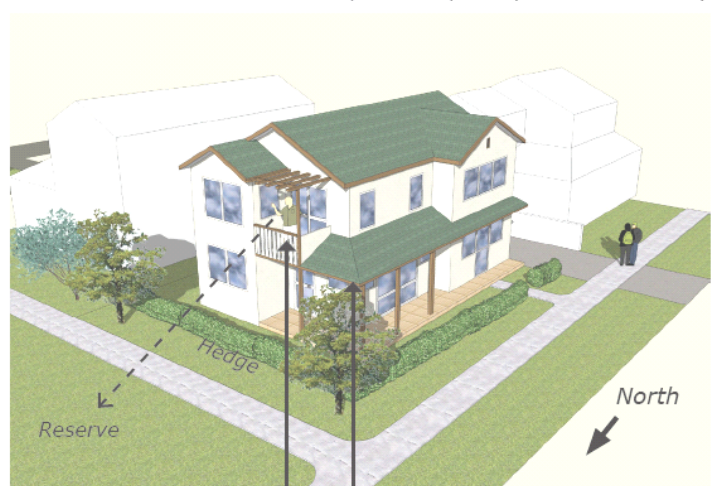
Illustration - house south of road and reserve using balcony and verandah as semi-private space (refer criterion 3)
