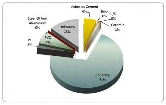
Figure 5.6 Pipes and Culvert Material Source: Auckland Council, June 2015
