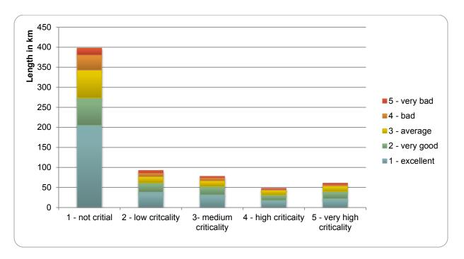
Figure 5.20 Condition by pipe asset criticality Source: Auckland Council, June 2015
