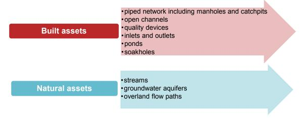
Figure 5.1 Stormwater assets
