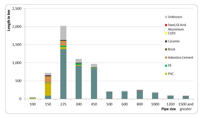
Figure 5.2 Pipe diameters, lengths and material Source: Auckland Council, June 2015
