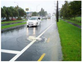
Figure 5.26 Surcharging Manhole, Northcote
