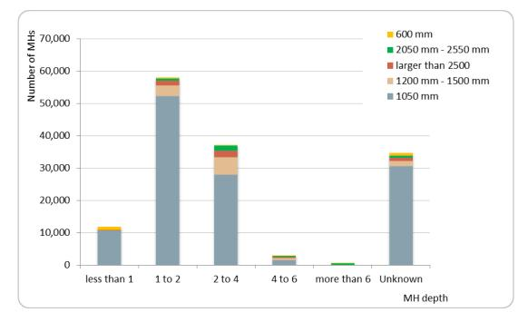
Figure 5.5 Manhole size and depth distribution Source: Auckland Council, June 2015
