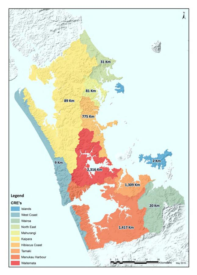
Figure 5.3 Lengths of pipes per CRE catchment Source: Auckland Council, June 2015
