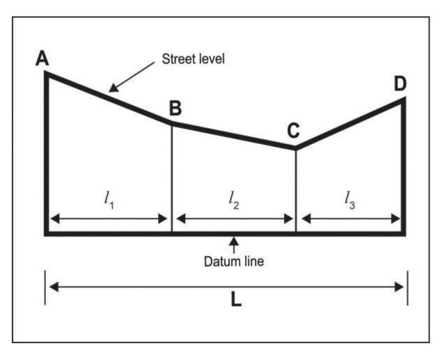
(A, B, C and D represent the street levels at given points where the street gradient changes. L represents the length of the boundary).
