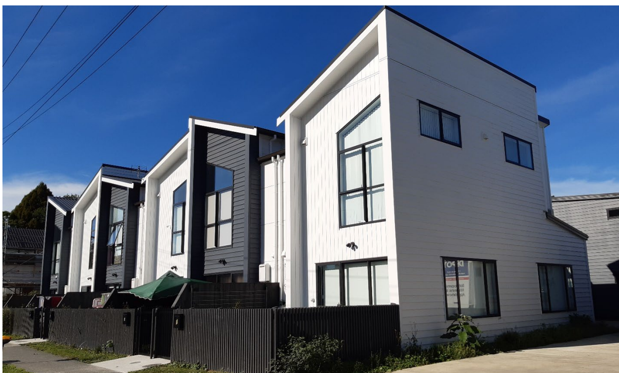
Figure 19. In this terrace development, the AUP outlook standard enables the principal living area outlook space to extend over the street boundary into the street space. The photo shows terraces with a 4m outlook space from the ground level living room within the site and a further 2 metres beyond the fence, extending into the street space. The close proximity to the street can affect privacy with residents sometimes choosing to draw their blinds or use other privacy measures. A benefit of the close proximity of the internal and outdoor living areas to the street is it can feel safer for pedestrians, knowing residents may be close by.
