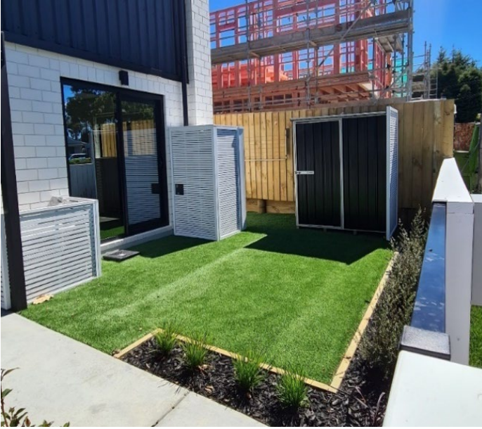
Figure 21: The useable space of the ground floor outdoor living area is reduced by the presence of a heat pump, shed and water tank. In this site, the items are screened. The useable space on the balcony in the apartment building is reduced by the external heat pump unit.
