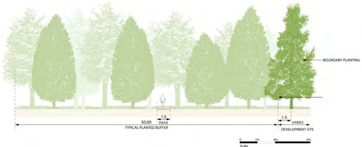
Diagram 5: Typical landscape buffer cross section
