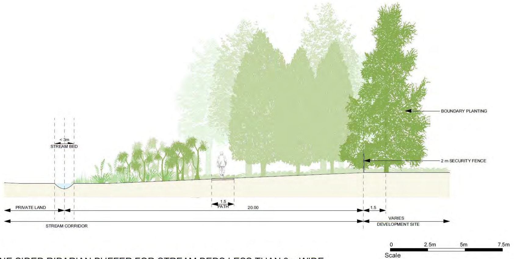
TYPICAL ONE SIDED RIPARIAN BUFFER FOR STREAM BEDS LESS THAN 3m WIDE
