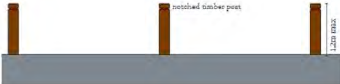
Figure 13 - Fencing Detail 3 - Public Open Space - Conservation
